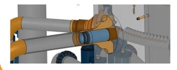
Model of the components of interest, including nozzle, sparger and feedwater lines
