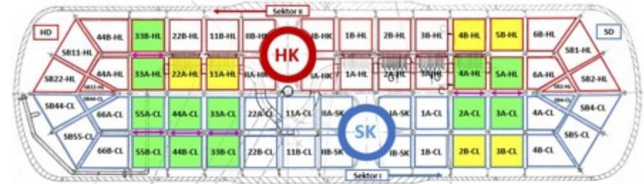
Limitations of the cleaning manipulator (pilot cleaning vs. subsequent cleaning)
