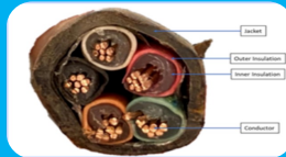
Cable Aging Management: Identification of Adverse Environment, & Introduction to Visual/Tactile Assessment of Cable
